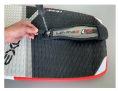
While holding back the nylon cover of the strap, insert one screw through the plastic washer into the screw insert of your choice. Tighten the screw firmly.
