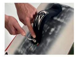
Insert the enclosed M6 counterhead bolt through the footstrap into the desired rear footstrap hole (see drawing on page 9) and tighten firmly using the Torx tool.
