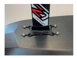
Position the mast plate of the assembled foil in alignment with the tracks on the bottom of the board. The leading edge of the mast should be pointing towards the nose of the board.
