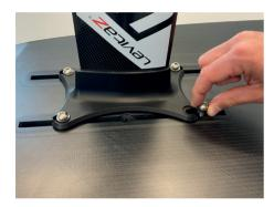
Slide the four bolts into the open fixing points of the mast plate and tighten the bolts, so that they are still able to slide in the tracks
