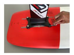
Slide the four bolts into the open fixing points of the the Board Adaptor and hand tighten the bolts that they are still able to slide in the tracks.
