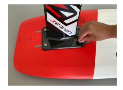
Insert the four bolts with its washers into the T-Nuts and hand tighten them.
