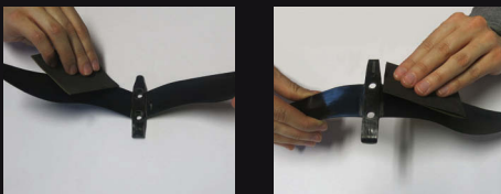
Pict. 2+3: Sharpening of the trailing edge
