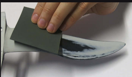
Pict. 5: Sanding the foil with a filler
