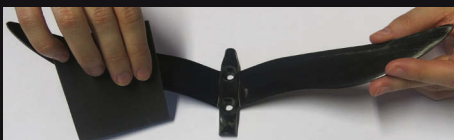
Pict. 4: Removing the burr of the leading edge
